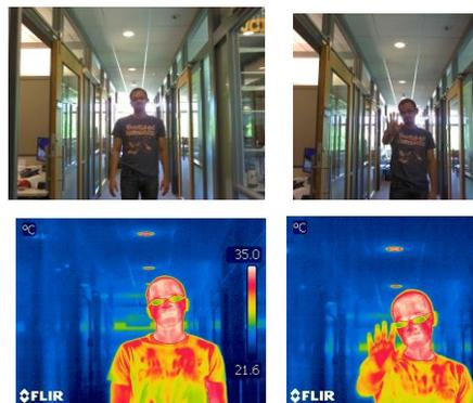
**Figure 4:** RGB images (top) vs. FIR images (bottom): The image on the right shows that a off-the-record gesture (trying to block the camera) can be also detected using an FIR image.
